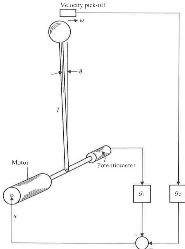
Figure 6.3 Implementation of system to stabilize inverted pendulum.
