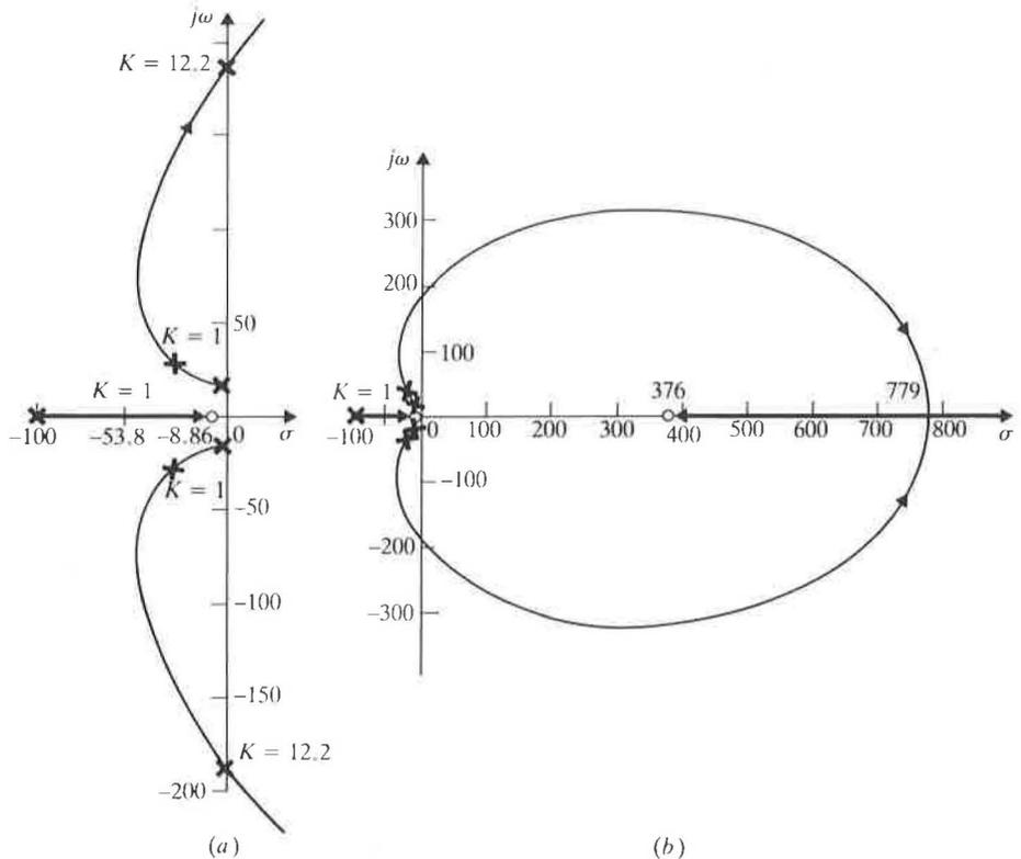
Figure 6.10 Root-locus plot for missile autopilot
