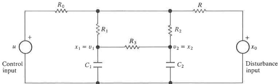
Figure 6.5 Electric network analog of temperature control problem.
