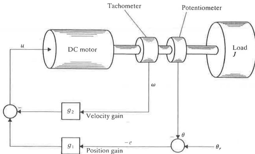
Figure 6.2 Implementation of an instrument servo.
