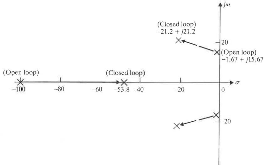
Figure 6.8 Open- and closed-loop poles for missile autopilot.
