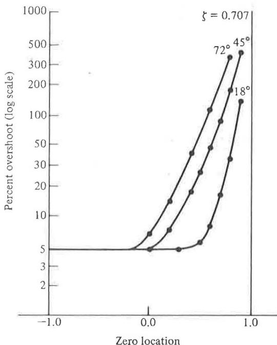
**Figure 2.31** Effects of extra zero on second-order system when  $\zeta = 0.707$ ;  $\theta = 18^\circ, 45^\circ, 72^\circ$ . Percent overshoot versus zero location.
