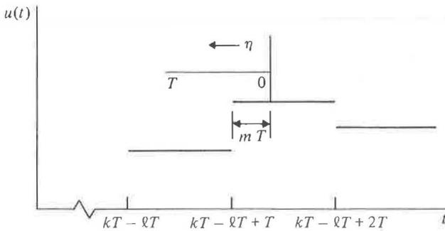
Figure 2.19 Sketch of a piecewise input and time axis for a system with time delay.
