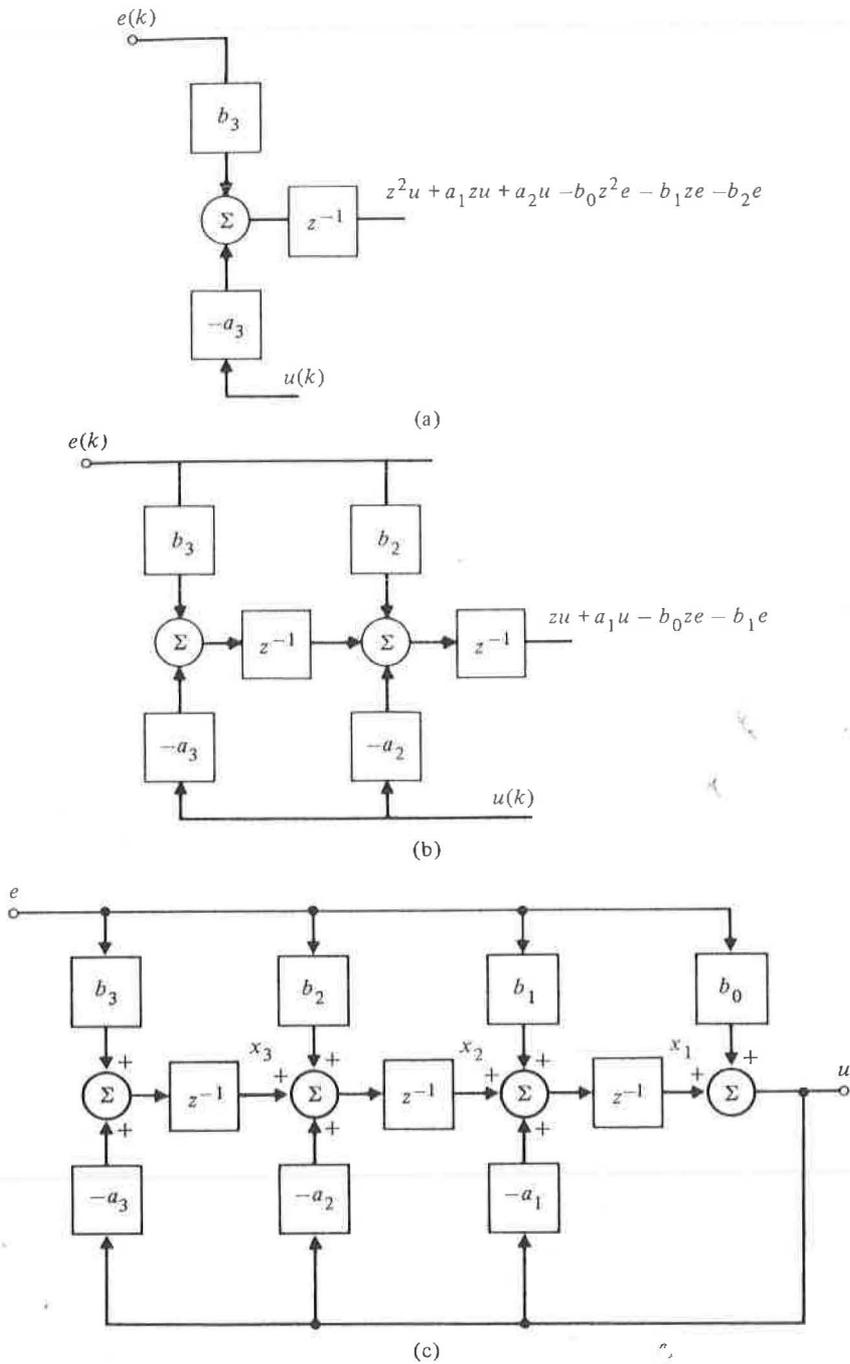
**Figure 2.9** Block diagram development of observer canonical form. (a) The first partial sum and delay; (b) the second partial sum and delay; (c) the completion with the solution for  $u(k)$ .
