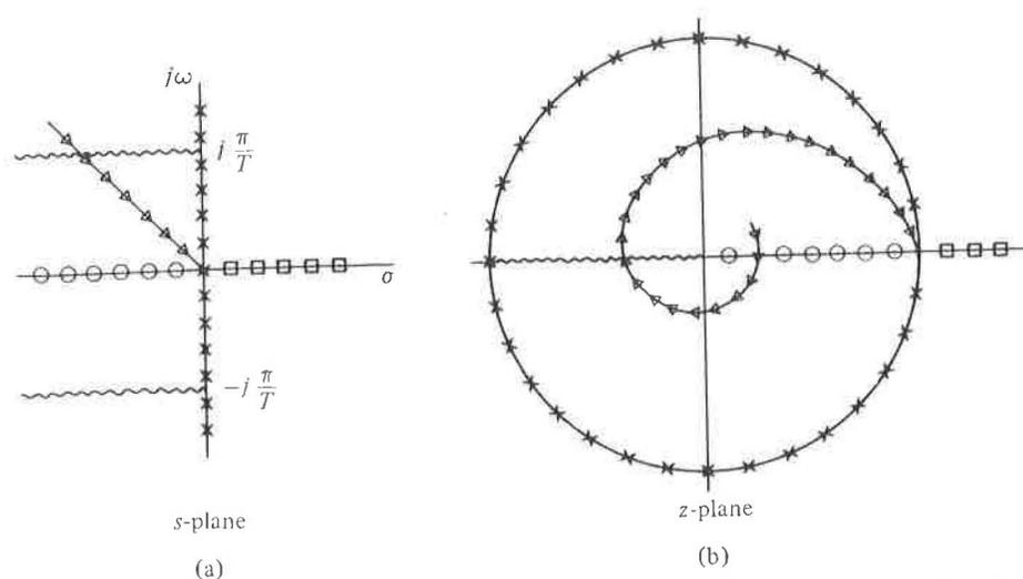
**Figure 2.26** Corresponding lines in the  $s$ -plane and the  $z$ -plane according to  $z = e^{sT}$ .
