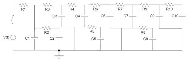
Initially, assume unit circuit elements. That is, the capacitors  $C_1,...,C_{10}=1F$ , the resistors  $R_1,...,R_{10}=1\Omega$  and voltage, V(t)=1V. At t=0, the switch is closed.
