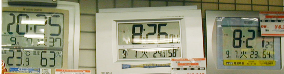
Fig. 1. What time is it? In this case the multisensor fusion problem is depicted by multiple clocks each giving different readings. The goal of estimation is to combine system knowledge to give the “best” final measure for the values of times and humidity in the room.
