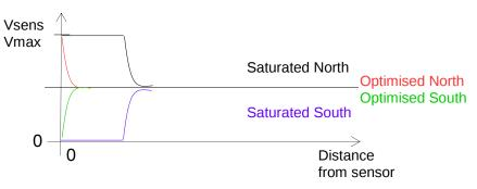
• From this graph you can see the relationship between distance and field strength (plus polarity) Use the data sheet to find magnet strength.
