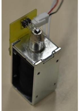
$\rightarrow$  It might help to wrap a piece of tape over the entire plunger and solenoid assembly
