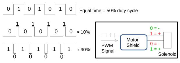
The PWM signal controls the polarity of the solenoid's magnetic field -i.e. 1 = north, 0 = south.
