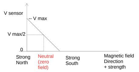
• you can measure the solenoid field strength by applying a known PWM value, then measuring the sensor voltage. Repeat this for all values up to 4095. This will give you this relationship between PWM and sensor voltage. (Something like the case below, but it may not map to these values)
