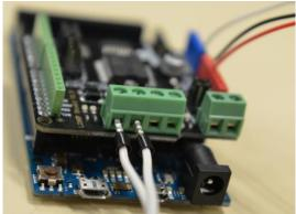
$\rightarrow$  Note that the solenoid is (by default) connected to the top or left pair. If you connect it to the righ, you'll have to update the software in several places.
