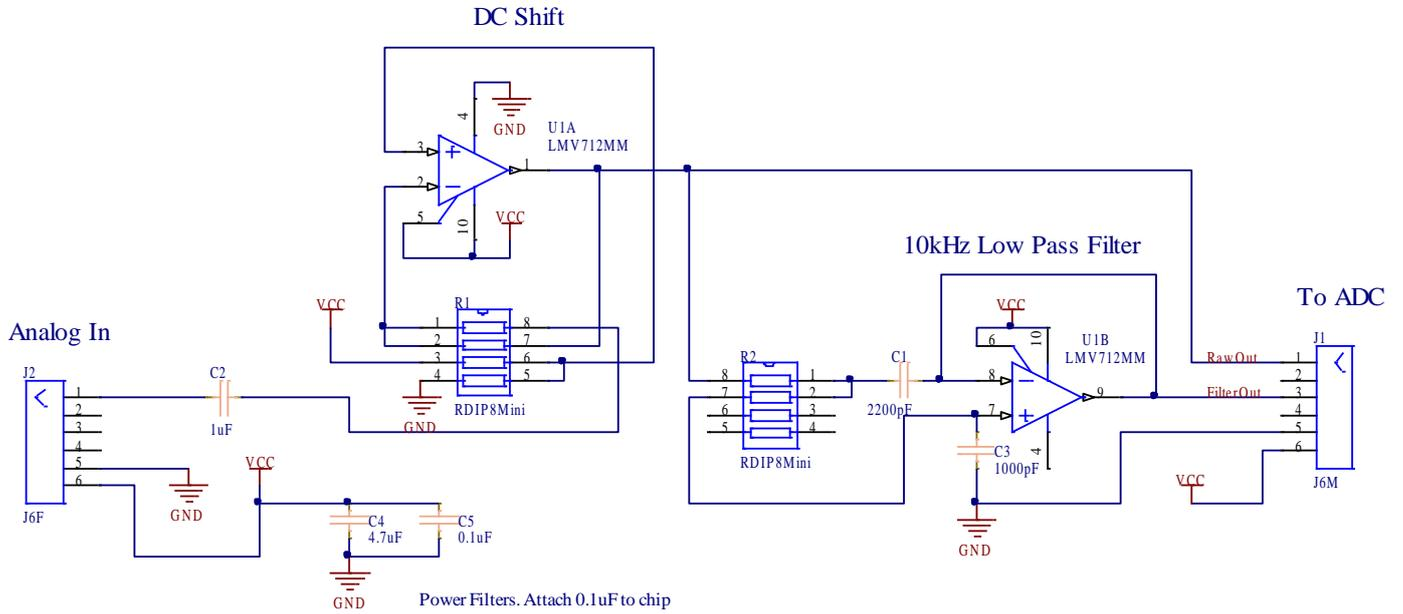
Figure 18 ADC lowpass filter
