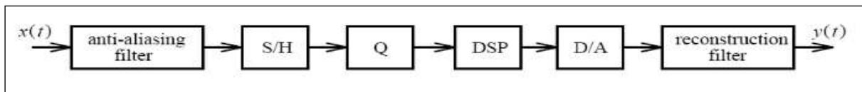
Figure 1. A block diagram of a practical DSP system
