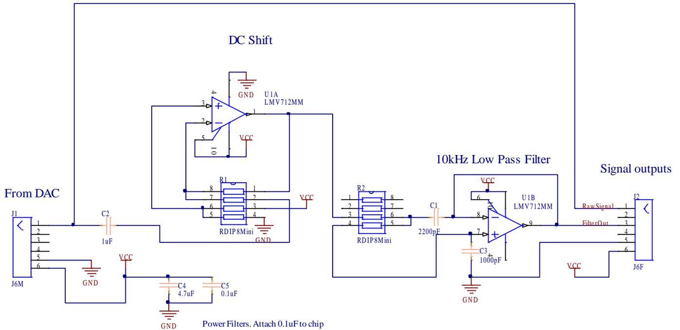
Figure 19 DAC lowpass filter
