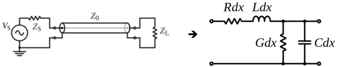
Giving:  $\frac{d^2 V(x)}{dx^2} + \omega^2 LC \cdot V(x) = 0$  and  $\frac{d^2 I(x)}{dx^2} + \omega^2 LC \cdot I(x) = 0$
