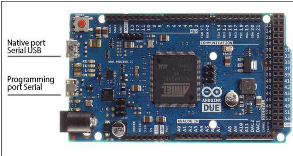
Figure 4 Arduino Due
