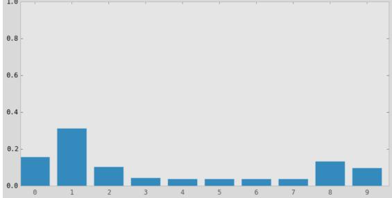
Notice the tall bar at position 1. This corresponds with the (correct) case of starting at position 0, sensing a door, shifting 1 to the right, and sensing another door. No other positions make this set of observations as likely. Now lets add an update and then sense the wall.
