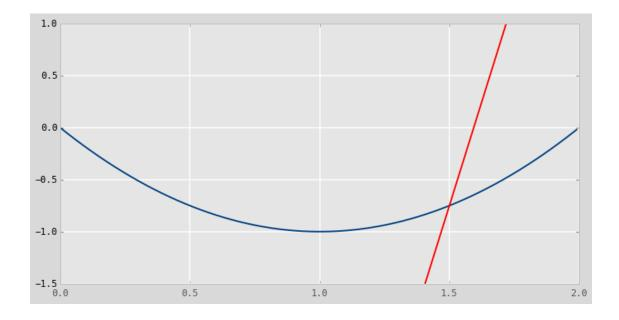
We can see that the linearization is exactly correct for x = 1.5, but very quickly diverges as x varies from 1.5. This does not constitute a proof that taking the derivative is a good linearization, but it should be fairly convincing.
