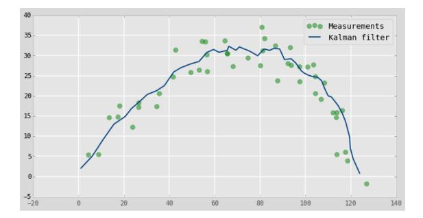
This output is terrible. The filter has no choise but to give more weight to the measurements than the process (prediction step), but when the measurements are noisy the filter output will just track the noise. This inherent limitation of the linear Kalman filter is what lead to the development of nonlinear versions of the filter.
