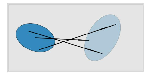
Here on the left we show an ellipse depicting the  $1\sigma$  distribution of two variables. The arrows show how three randomly sampled points might be transformed by some arbitrary nonlinear function to a new distribution. The ellipse on the right is drawn semi-transparently to indicate that it is an *estimate* of the mean and variance of this collection of points - if we were to sample, say, a million points the shape of the points might be very far from an ellipse.
