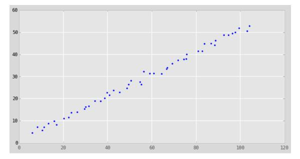
That looks correct. The slope is 1/2, as we would expect with a velocity of (2,1), and the data seems to start at near (6,4).
