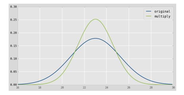
The result is either amazing or what you would expect, depending on your state of mind. I must admit I vacillate freely between the two! Note that the result of the multiplication is taller and narrow than the original Gaussian but the mean is the same. Does this match your intuition of what the result should have been?
