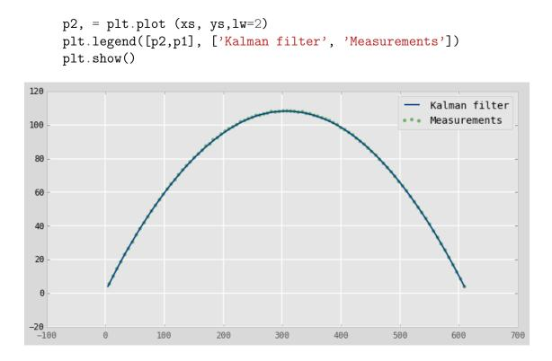
We see that the Kalman filter reasonably tracks the ball. However, as already explained, this is a silly example; we can predict trajectories in a vacuum with arbitrary precision; using a Kalman filter in this example is a needless complication.
