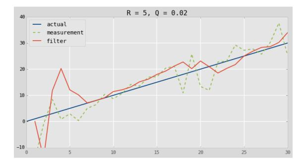
The filter in the first plot should follow the noisy measurement almost exactly. In the second plot the filter should vary from the measurement quite a bit, and be much closer to a straight line than in the first graph.
