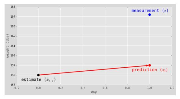
Here the measurement is in blue, the previous estimate (output of the filter) is black, and the estimate is red. So we have a problem. Our prediction doesn't match our measurement. But, that is what we expected, right?. If the prediction was always exactly the same as the measurement, it would not be capable of adding any information to the filter.
