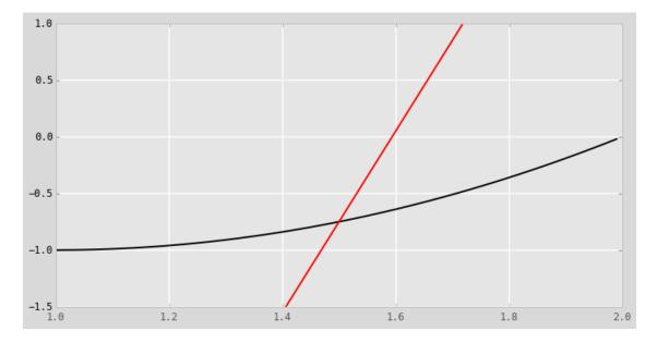
This is not a good linearization for f(x). It is exact for x = 1.5, but quickly diverges when x varies by a small amount.
