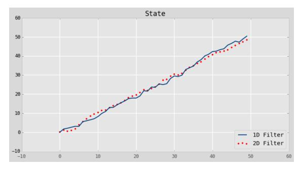
**Discussion** The output of the filter that incorporates velocity into the state produces much better output than the filter that only tracks position - the output is much closer to a straight line. We've already discussed why unobserved variables increase the precision of the filter, so I will not repeat that explanation here. But the last exercise and this one is intended to trigger a train of thought:
