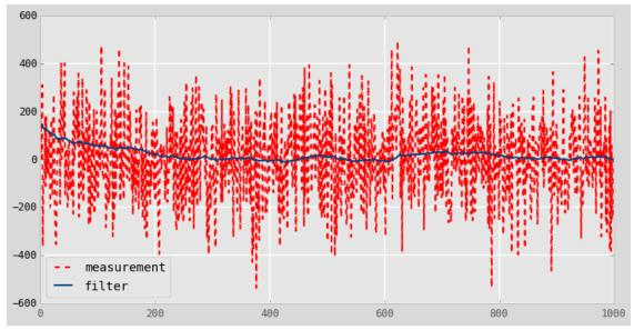
This simple change significantly improves the results. On some runs it takes 200 iterations or so to settle to a good solution, but other runs it converges very rapidly. This all depends on whether the initial measurement Z had a small amount or large amount of noise.
