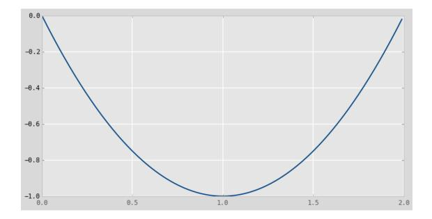
Suppose we want to linearlize this equation so we can evaluate it's value at 1.5. In other words, we want to create a linear function of the form  $y_l(x) = ax + b$  such that  $y_l(1.5)$  gives the same value as y(1.5). Obviously there is not single linear equation that will do this. But if we linearize y(x) at 1.5, then we will have a perfect answer for  $y_l(1.5)$ , and a progressively worse answer as our evaluation point gets further away from 1.5.
