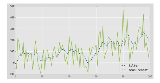
This doesn't look so wonderful to me. We can see that perhaps the filtered signal varies less than the noisy signal, but it is far from the straight line. If we were to plot just the filtered result no one would guess that the signal with no noise starts at 5 and increments by 2 at each time step. And while in locations the filter does seem to reduce the noise, in other places it seems to overshoot and undershoot.
