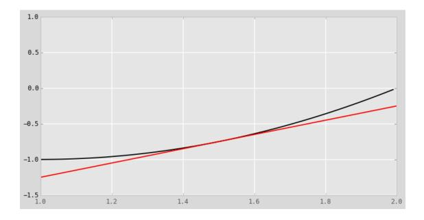
Here we can see that this linearization is much better. It is still exactly correct at x = 1.5, but the errors are very small as x varies. Compare the tiny error at x = 1.4 vs the very large error at x = 1.4 in the previous plot. This does not constitute a formal proof of correctness, but this sort of geometric depiction should be fairly convincing. Certainly it is easy to see that in this case if the line had any other slope the errors would accumulate more quickly.
