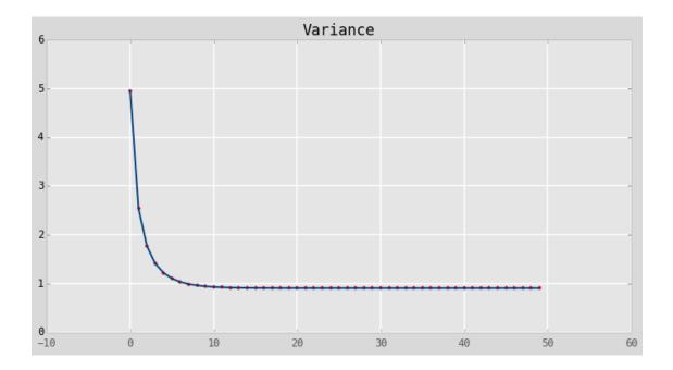
**Discussion** As you can see, both filters produce the same results. Feel free to vary the initial guess, the measurement noise, and the process noise; so long as you make the same changes to both filters the output should be the same. This is a solid demonstration, albeit not a rigorous proof, that both filters in fact implement the same math for the 1-D case.
