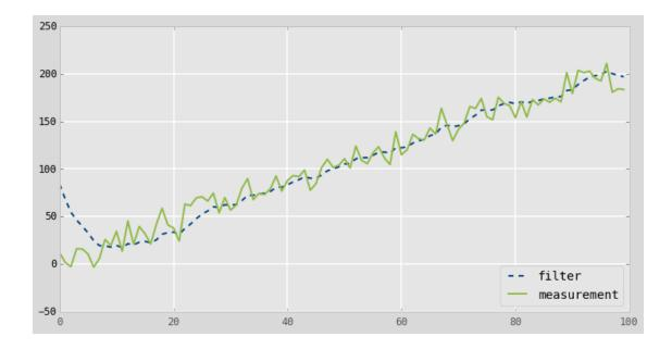
The filter starts out with estimates that are far from the measured data due to the bad initial guess of 100. You can see that it 'rings' before settling in on the measured data. 'Ringing' means that the signal overshoots and undershoots the data in a sinusodial type pattern. This is a very common phenomena in filters, and a lot of work in filter design is devoted to minimizing ringing. That is a topic that we are not yet prepared to address, but I wanted to show you the phenomenon.
