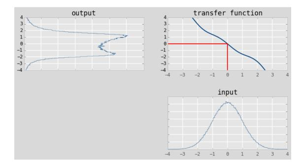
This result may be somewhat suprising to you. The transfer function looks "fairly" linear - it is pretty close to a straight line, but the probability distribution of the output is completely different from a Gaussian. Recall the equations for multiplying two univariate Gaussians:
