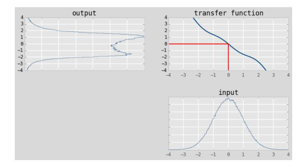
I generated this by taking 500,000 samples from the input, passing it through the nonlinear transform, and building a histogram of the result. From that histogram we can then compute a mean and a variance that we compared to the output of the EKF.
