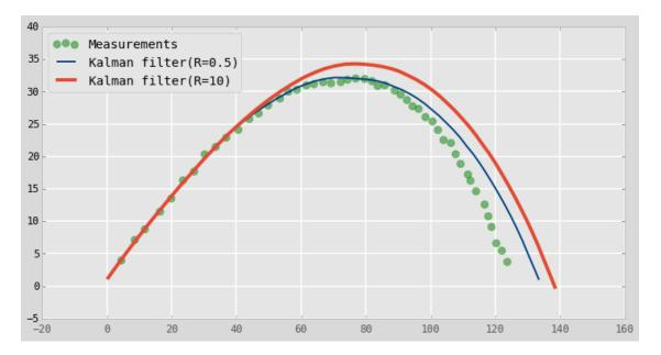
I have plotted the output of two different Kalman filter settings. The measurements are depicted as green circles, a Kalman filter with R=0.5 as a thin blue line, and a Kalman filter with R=10 as a thick red line. These R values are chosen merely to show the effect of measurement noise on the output, they are not intended to imply a correct design.
