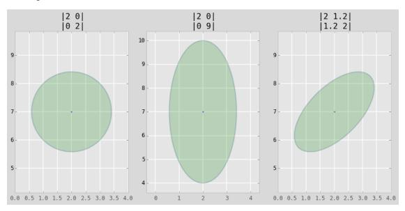
From a mathematical perspective these display the values that the multivariate gaussian takes for a specific standard deviation (in this case  $\sigma = 1$ ). Think of it as taking a horizontal slice through the 3D surface plot we did above. However, thinking about the physical interpretation of these plots clarifies their meaning.
