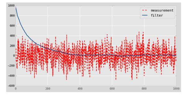
This time the filter does struggle. Notice that the previous example only computed 100 updates, whereas this example uses 1000. By my eye it takes the filter 400 or so iterations to become reasonable accurate, but maybe over 600 before the results are good. Kalman filters are good, but we cannot expect miracles. If we have extremely noisy data and extremely bad initial conditions, this is as good as it gets.
