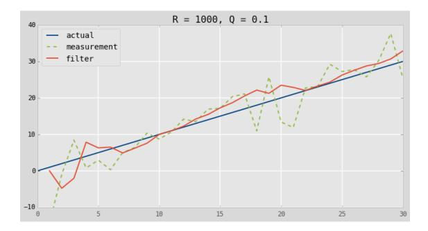
The filter output should be much closer to the green line, especially after 10-20 cycles. If you are running this in Ipython Notebook, I strongly urge you to run this many times in a row (click inside the code box, and press CTRL-Enter). Most times the filter tracks almost exactly with the actual position, randomly going slightly above and below the green line, but sometimes it stays well over or under the green line for a long time. What is happening in the latter case?
