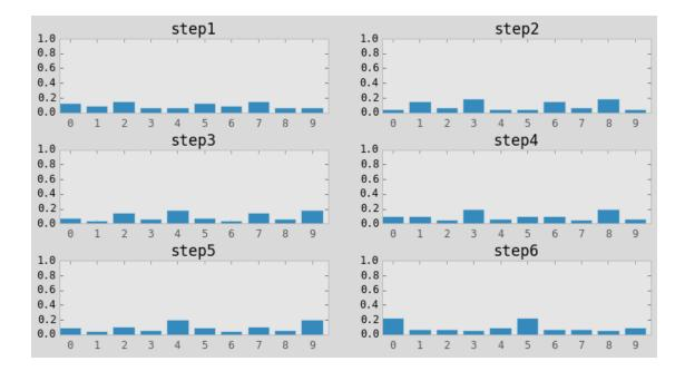
As you can see we quickly filtered out the bad sensor reading and converged on the most likely positions for our dog.
