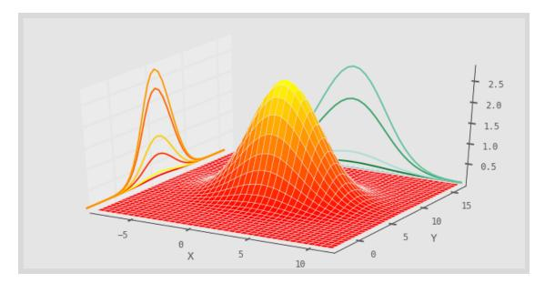
The result is clearly a 3D bell shaped curve. We can see that the gaussian is centered around (2,7), and that the probability quickly drops away in all directions. On the sides of the plot I have drawn the Gaussians for x in greens and for y in orange.
