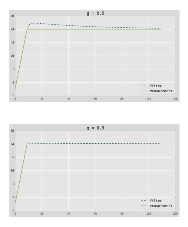
Here we can see the effects of ignoring the signal. We not only filter out noise, but legitimate changes in the signal as well.
