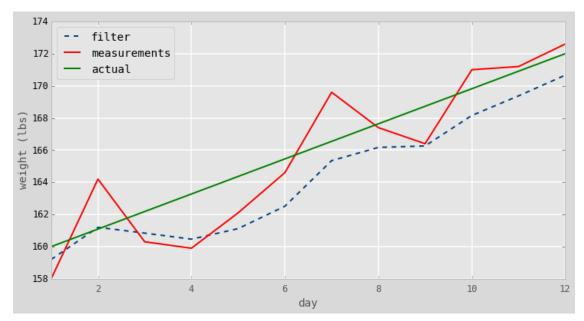
Clearly a filter that requires us to correctly guess a rate of change is not very useful. Even if our initial guess was useful, the filter will fail as soon as that rate of change changes. If I stop overeating the filter will have extremely difficulty in adjusting to that change.
