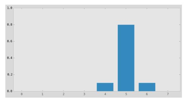
The simple test case that we ran appears to work correctly. We initially believed that the dog was in position 3 with 100% certainty; after the movement update we now give an 80% probability to the dog being in position 5, and a 10% chance to undershooting to position 4, and a 10% chance of overshooting to position 6. Let us look at a case where we have multiple beliefs:
