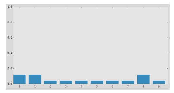
We can see that this is not a probability distribution because it does not sum to 1.0. But we can see that the code is doing mostly the right thing - the doors are assigned a number (0.12) that is 3 times higher than the walls (0.04). So we can write a bit of code to normalize the result so that the probabilities correctly sum to 1.0.
