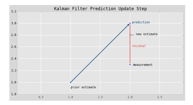
The blue point labeled "prediction" is the output of  $\mathbf{Hx}$ , and the dot labeled "measurement" is  $\mathbf{z}$ . Therefore,  $\gamma = \mathbf{z} - \mathbf{Hx}$  is how we compute the residual, drawn in red, where  $\gamma$  is the residual.
