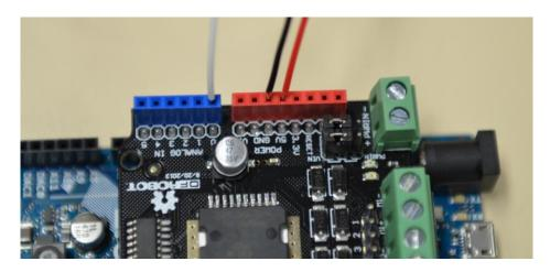
**Step 9: Connect the Solenoid Actuator to the Arduino**
