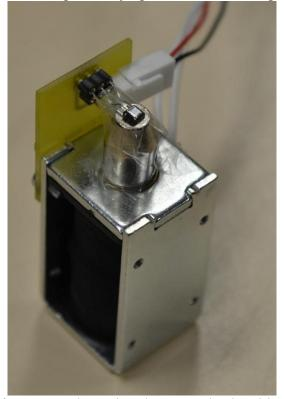
→ It might help to wrap a piece of tape over the entire plunger and solenoid assembly
