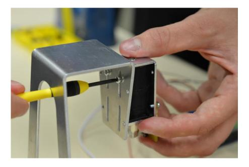
Step 8: Connect the Hall-Effect Sensor to the Arduino
