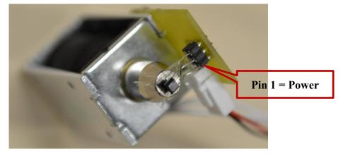
→ Remember to add tape to the top of the plunger before adding the sensor.
