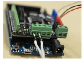
→ Note that the solenoid is (by default) connected to the top or left pair. If you connect it to the righ, you'll have to update the software in several places.
