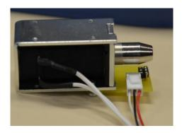
**Step 3: Add (Electrical) Tape to Insulate the Hall-Effect Sensor from the Electromagnet**Put a piece of tape onto the top of the electromagnet as shown. This is an important step for later, as if the magnet accidentally collides with the sensor, the sensor leads will press against the plunger, causing a short
