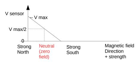
• For activity 1, you can measure the solenoid field strength by applying a known PWM value, then measuring the sensor voltage. Repeat this for all values up to 4095. This will give you this relationship between PWM and sensor voltage.
