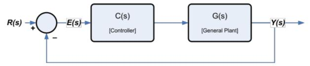
Recall that the first method is particularly apt for systems that can be approximated as a first-order plant having a transport **delay** (L) and **rise slope** (K/ $\tau$ ), thus  $G(s) = \frac{Ke^{-Ls}}{\tau s+1}$
