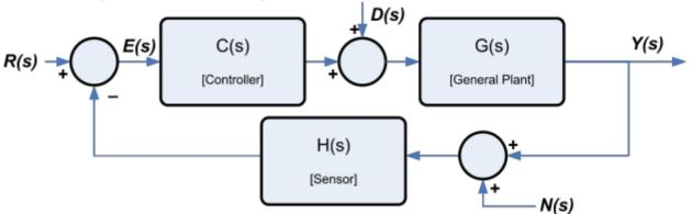
For such a system, we can define the **Loop Gain**, **L(s)**:
