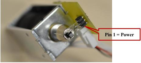
$\rightarrow$  Remember to add tape to the top of the plunger before adding the sensor.
