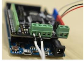
$\rightarrow$  Note that the solenoid is (by default) connected to the top or left pair. If you connect it to the righ, you'll have to update the software in several places.
