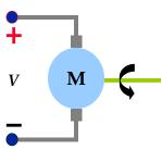
Recall that the torque is given by  $\tau = ki$ . The mechanical torque model is given by  $I\omega' = -b\omega + \tau$
