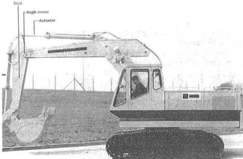
Figure 5.38 An excavator with an automatic control system.
